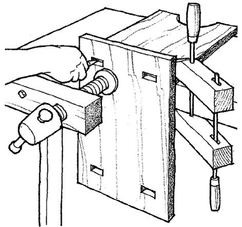
**Step 5:** Extend tenon layout lines down the face of the stock with a square.
