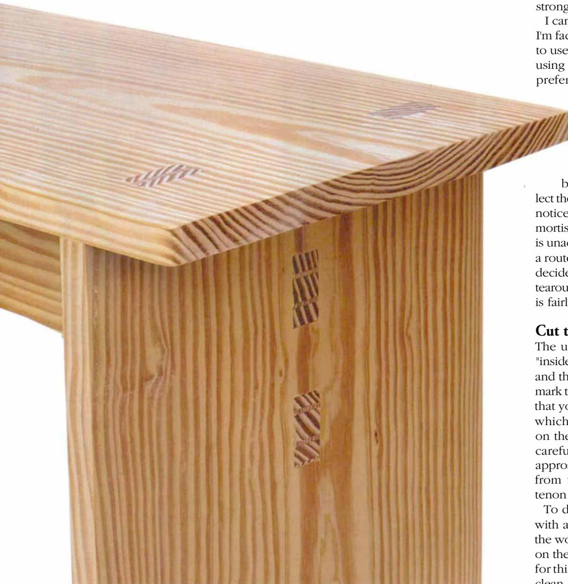
*Work carefully when joinery is exposed. The author cuts mortises first and then marks the tenons to reduce tearout on the face side.*
