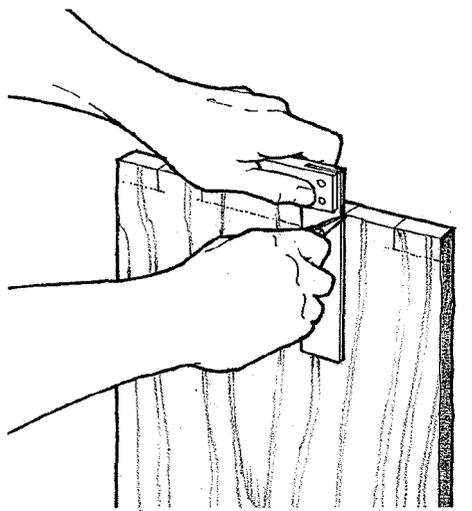
**Step 6:** Mark the length of the tenons with a marking gauge or knife, and then cut to the line on a bandsaw.
