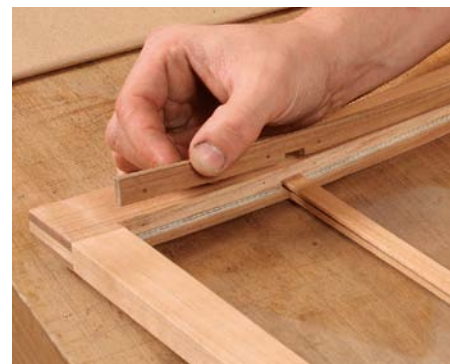
Add the stops. They were cut from the rails earlier. Drill clearance holes for the pins that hold them in place. Push them in with a wood block, protecting the glass with cardboard.
