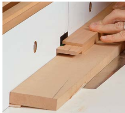
A shim does it. A shim glued to the underside of a piece of MDF lets you rout the angled rabbets with a straight bit.
