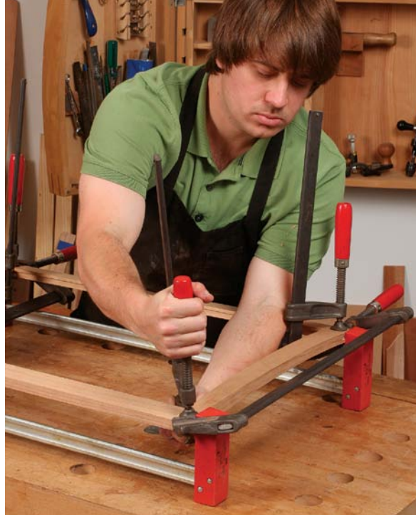
Clamp bridle joints from three directions. Go across the width and down the length and then add a clamp to press the sides of the slot tight against the tenon.
