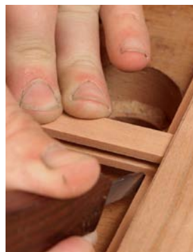
Fine-tune the fit. Dry-fit the mullions and mark for a notch that brings them flush with the front of the rails.
