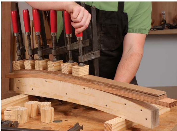
Spread the pressure evenly. Kellogg uses blocks under the clamp head and three hardboard cauls to ensure that all of the glue joints are tight.
