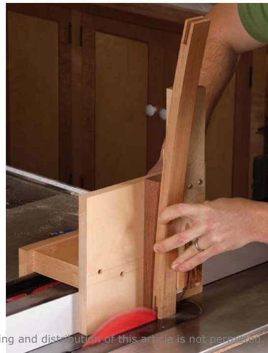
Cut the slots at the table-saw. Add a cradle to your tenoning jig, curved to match the rail, to hold the rail at the correct angle.
