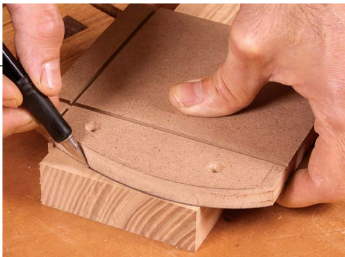
Template for the end. While the workpiece is still square, use the template's fence for alignment. It registers against the bottom edge, so the same section of curve is used for all eight ends. Lay out the curve and then cut it.
