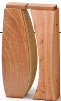
A pair of these blocks gives you a straight edge for layout and clamping, and a curved one that helps you chop perfect shoulders.
