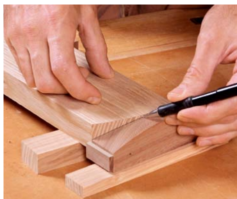
Block for the curved faces. A fence on the block aligns it with the bottom edge (left). The shim under the block is the same thickness as the workpiece's final thickness. Remove the shim to trace the inside face (right).
