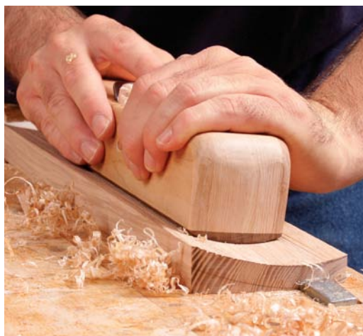
Clean it up with plane. You'll need one with a radiused bottom tighter than the tightest part of the curve. Roy made his, but you can buy new and used "round" molding planes from a variety of sources.
