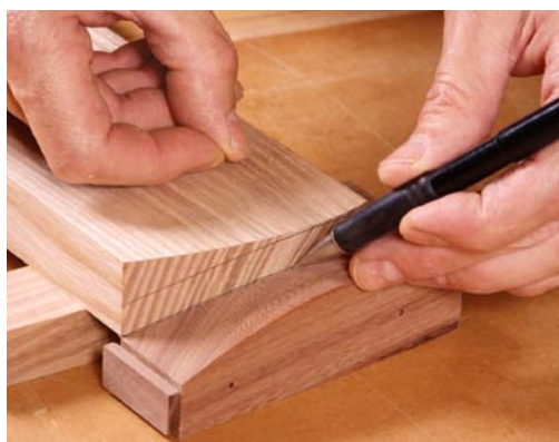
Block for the curved faces. A fence on the block aligns it with the bottom edge (left). The shim under the block is the same thickness as the workpiece's final thickness. Remove the shim to trace the inside face (right).
