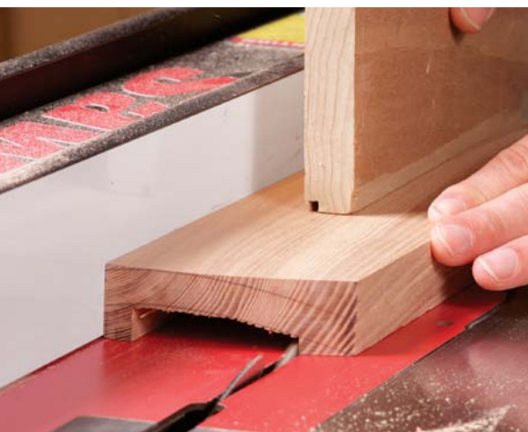
Rough out the inside curve first. Make a series of ripcuts. Keep the blade square to the table and adjust its height so that each cut is just shy of the layout line.
