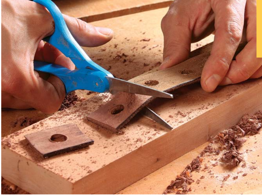
Prep the washers. After scraping the leather clean and drilling \frac{1}{2} -in. holes into it, Tetreault uses a sturdy pair of scissors to cut out the washers.
