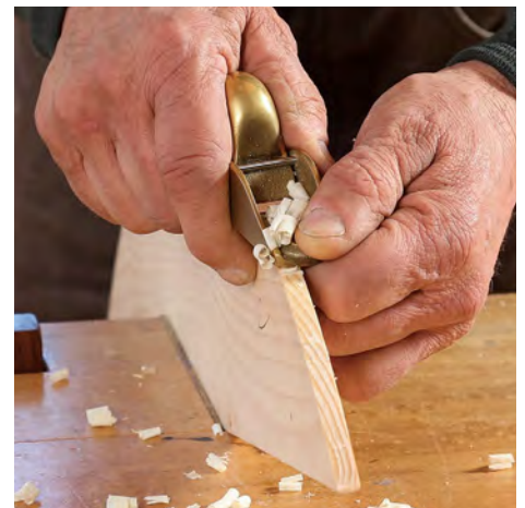
Don't forget the block plane. In fact, have two: a small one like a violin maker's plane for coarse work and convex curves (shown), and an adjustable-mouth block plane for fine work.
