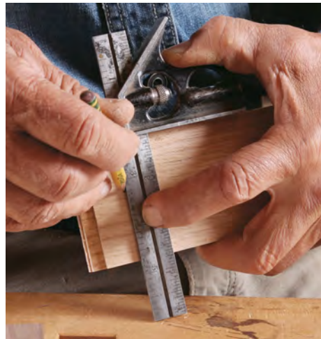
One tool, many jobs. A combination square can be used for layout, checking joints for accuracy, setting up machinery, transferring measurements, and a host of other jobs.
