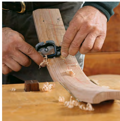
Flat-sole spokeshave for curves. Hack prefers one with an adjustable mouth and a cambered blade. No other tool handles both convex and concave curves as well.
