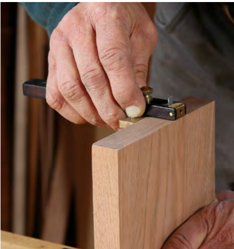
You need marking gauges. It's the right tool for laying out dovetails and tenon shoulders. You can lay out tenon cheeks with one, but you must change the setting. Two gauges makes it easier.
