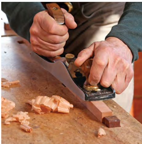
One bench plane is all you need. A low-angle jack plane, along with an extra blade cambered for smoothing, can do everything from jointing to smoothing. And because it lacks a frog, it weighs less than a standard jack plane.
