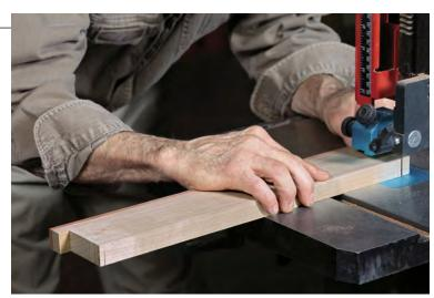
**Trim the waste.** Cut the stub tenon to length and the dovetail to width. Neptune uses a bandsaw and cleans to the line with a chisel.
