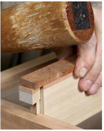
**Tap in the divider.** Use a scrap block to protect the workpiece as you drive the divider into the case.
