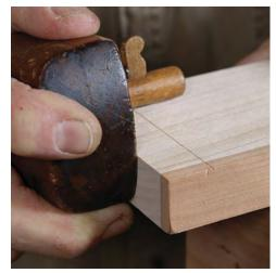
**Scribe the shoulders.** Set the divider in place and check that the dovetail shoulders align with the inside of the case (right).
