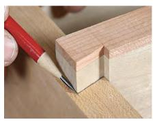
Trace the dovetail onto the case side.
