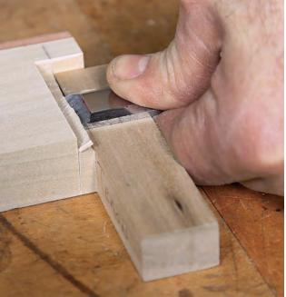
Flat block ensures consistent tenons. Establish the shoulder with heavy vertical cuts, staying inside the scribe line (above). Then follow with careful cuts to the line. Use the paring block (left) to cut the stub tenon to thickness. Start by roughing out the bulk of the waste. For the final cuts, keep the back of the chisel pressed firmly against the paring block and take narrow shavings.
