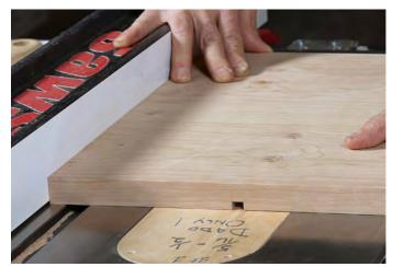
The dado size depends on which dovetail you pick. If you are making a stepped-dovetail divider and your dado stack's outside blades leave deeper scoring marks, level the bottom of the case dadoes with a router plane. Otherwise, the show face of the joint will have triangular gaps at the shoulder.
