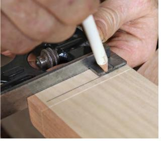
Determine stub tenon length. With the divider still in place, pencil the dado depth on the divider (above). This will be the length of the stub tenon. Use a combination square to carry the line across the divider (left).
