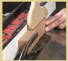
**Rip the block.** Saw the ramp, then smooth it with a handplane. Neptune bandsaws flats on each end of the paring block to create surfaces for clamping.
