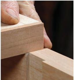
Mark the dovetail length. The shoulder of the tail should align with the bottom of the dado. Neptune sneaks up on this dimension with a marking gauge at the back edge of the divider to keep the show edge clean.
