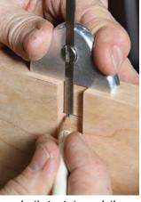
**Mark the dovetail and housing.** Use a depth gauge to mark the width of the dovetail both on the divider and the case side.
