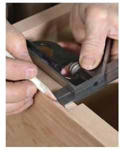
Lay out the dovetail housing. Use a combination square to mark the length of the dovetail on each case side.
