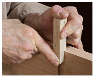
**Size the tenon paring block.** Plane this block so it's a tight press-fit in the dado.
