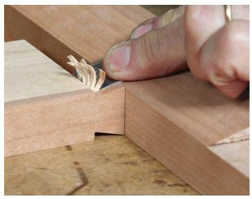
**Pare the dovetail with angled paring block.** Flip the board to pare both faces. Remove most of the waste before taking careful finishing cuts.
