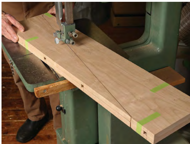
Dadoes first. Before tapering the sides, cut three dadoes per side. Becksvoort uses a miter gauge and the fence with a dado blade.
