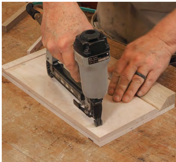
Small flats on fence and base mitered ends allow for easy alignment when assembling the shooting board.
