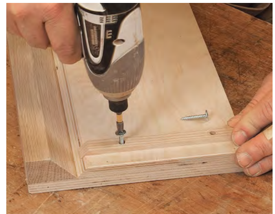
Add the stop. The stop acts as a zero-clearance support and prevents chipout when planing. It gets worn out over time, but oversize holes allow for adjustment for a fresh cut on occasion.
