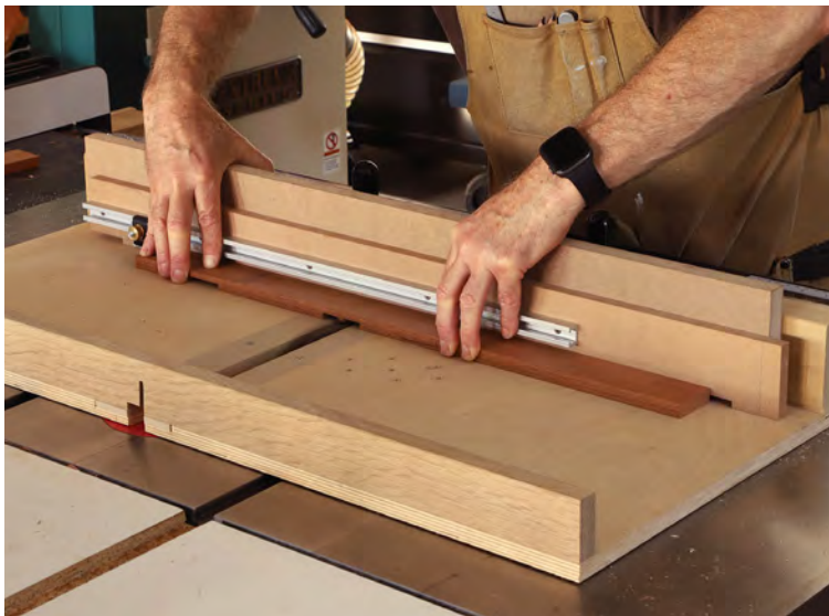
Upper level box joints. To cut the half-laps, Hartman made a variation on a box-joint jig, with an indexing pin to control the cuts. But his jig has a “crenellation board” with wide notches in the bottom edge and a stop on the front. The workpiece moves laterally with the crenellation board, and the notches fit over the pin. Each half-lap is cut in three passes.
