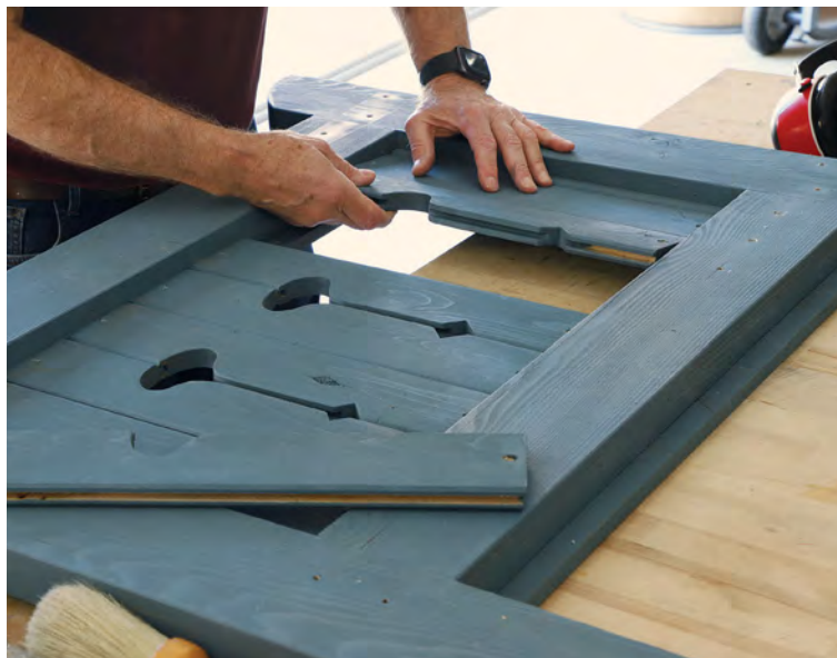
Creating the cutouts. Hartman sets the scroll-sawn tongue-and-groove slats in place, adding spacers on either side to even the spacing, if necessary.
