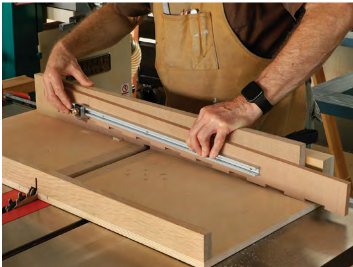
Upper level box joints. To cut the half-laps, Hartman made a variation on a box-joint jig, with an indexing pin to control the cuts. But his jig has a “crenellation board” with wide notches in the bottom edge and a stop on the front. The workpiece moves laterally with the crenellation board, and the notches fit over the pin. Each half-lap is cut in three passes.
