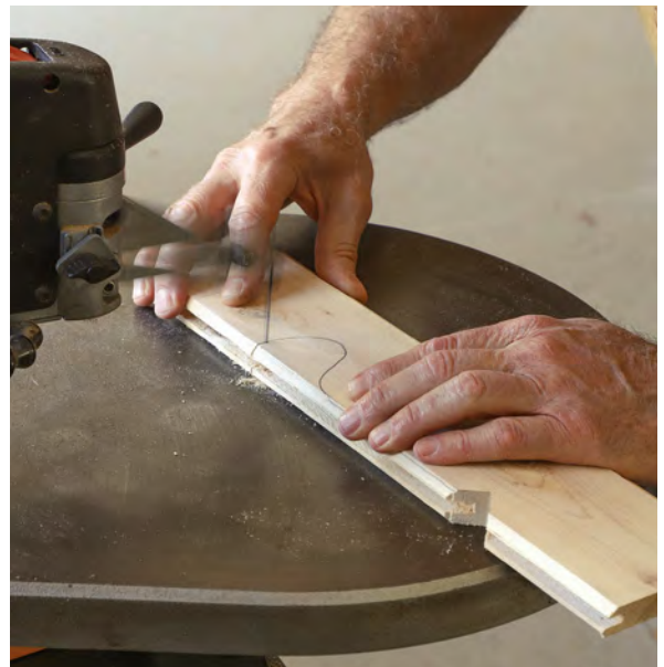
Panel parts. Mating panel slats get cutouts sawn on the scroll saw.
