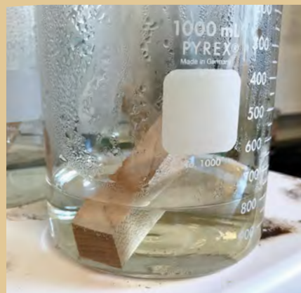
Extractives can be transported by water. Extractives can be transferred to humans either through dust breathed in when milling or sanding, or via contact with skin, food, or saliva. And water can transfer extractives. After being boiled for 30 minutes, the water around a block of hard maple (left) is clear, due to the wood's relative lack of extractives. The same test conducted on walnut (right), which has more extractives, turns water brown.
