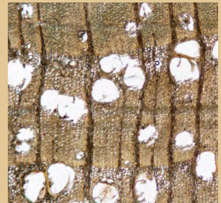
Tropical woods have more extractives. Teak, found throughout Asia, Africa, and the Caribbean, contains a number of extractives that produce its dark color and oily feel. These characteristics are evident on the surface of a board (left). In a magnified cross-section (right), all of the brown color and tinting are extractives.
