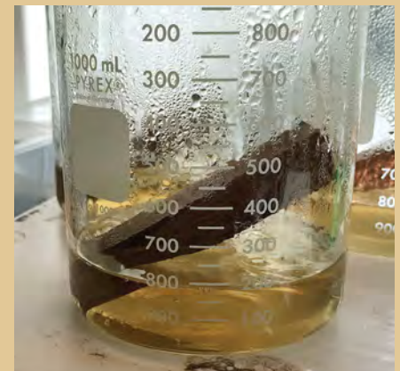
Extractives can be transported by water. Extractives can be transferred to humans either through dust breathed in when milling or sanding, or via contact with skin, food, or saliva. And water can transfer extractives. After being boiled for 30 minutes, the water around a block of hard maple (left) is clear, due to the wood's relative lack of extractives. The same test conducted on walnut (right), which has more extractives, turns water brown.
